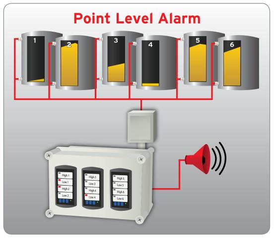
as a vessel is emptied or comes back into contact with the level indicator as a vessel is filled, the LED on the panel goes out altogether and the panel automatically resets – and is ready to receive the next alarm signal.
