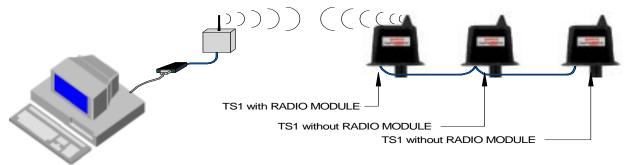
**NOTE:** There can be only **one** TS1 unit having a wireless modem connected to each wired RS-485 network. Do not connect multiple TS1 units with wireless modems to the same RS-485 network.
