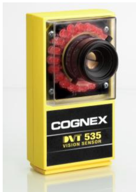
Figure 1: Member of The DVT Product Family: the DVT 535 Vision Sensor.
