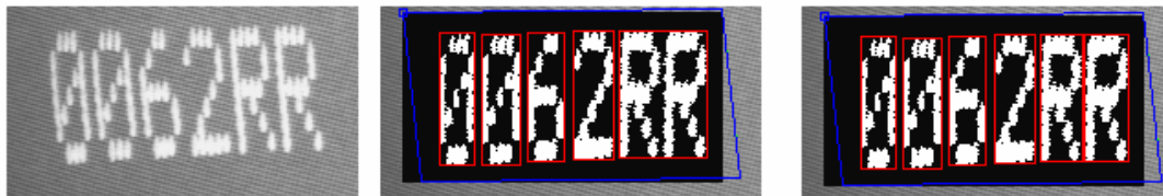
Figure 48: Use of the extraction tools to separate individual characters.
