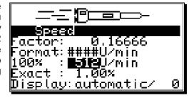
**Example:** With a 100% value of 512 rot/min you need to divide through 64, which corresponds to a shifting operation of SRW 6.
