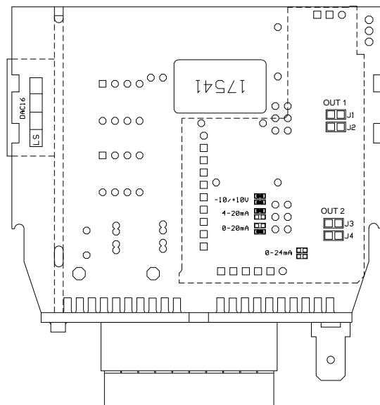
If you want to change the signal level, the device has to be opened. The case can be opened in the middle using a screwdriver. On the soldering side of the largest printed circuit board two soldering bridges for every analog output, i.e. the analog output 1(OUT1) and 2 (OUT2), are located, which are named J1 to J4 in the drawing to the right. J1 and J2 are used to adjust the signal level for output 1 and J3 and J4 to adjust the output level for output 2.
