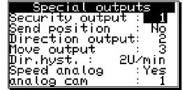
a single output, so that this output is switched off at the occurence of a mistake and serves as a security output. With a program change, the security output is reset for a short time (see chapter "7.4.6.6. Setting the program selection mode" on page 56).
