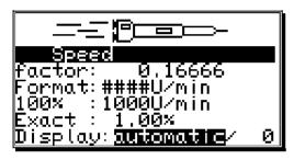
If you want to prevent the automatic switching at the 5% of the maximum speed in the "**Display**" menu point, you can select one of the three different display types with the key and the key.
