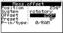
The offset is subtracted from the physical position. This makes it possible for you to shift the zero point.
