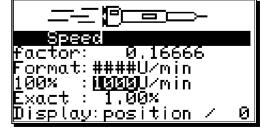
entered value, for 1000 rotations per minute it lies at 50 rotations per minute. Press the CR key or the key to move the cursor to the next menu point "Exact".
