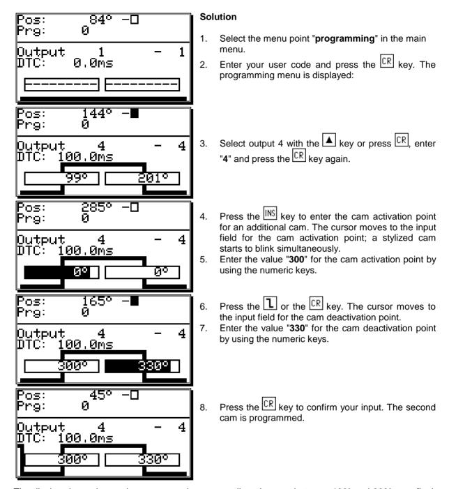
The display shows the newly programmed cam as well as the cam between 100° and 200° as a flank on the left edge of the display.
