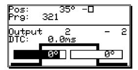
After you confirm your selection with the CR key, the field for the cam deactivation point is underlayed in black. Simultaneously, the dropping flank of the stylized cam starts to blink.
