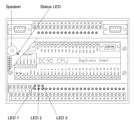
Additionally, CamCon DC90 is equipped with 3 other status LED. They are:
