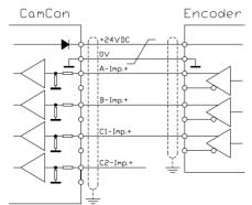
If a 24V PNP signal is used as a data input, you may only connect the (+) signals of the inputs. The (-) signals have to remain unswitched in this case. The connection of such a measuring system requires a change of the internal circuits and has to be specified with your order.
