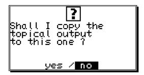
Move the cursor to "**yes**" with the key and press the Rey key to confirm your input. This starts the copying process. After a short while the new output will appear on the display.
