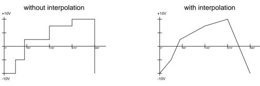
Through interpolation of the definition points, CamCon can adjust the values and present a curve, corresponding to the above right drawing.
