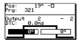
Here you can enter the positions for the activation and the deactivation point for the cam, as is described in the chapter "7.3.5. Cam Input". If you enter a cam that overlaps with an already existing cam, you create a single, greater cam.
