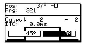
Enter the value for the cam deactivation point with the numeric keys and finish your input with the pressing of the CR key.
