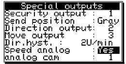
CamCon emitts a voltage (proportional to the speed) on the first analog output (pin 2 at CamCon DC50), 0 to -10V with a negative rotation direction and 0 to +10V with a positive rotation direction, if the menu point "Speed Analog" is set to "yes".
