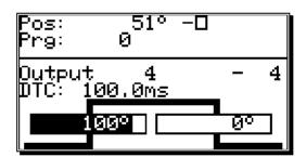
If you now press the key or the key, all the cams of this output are shifted by one increment. In this case the cams are directly taken over into the memory without the use of the CR key (unlike before). The shifting process is ended by pressing either the CR key or the ESC key.
