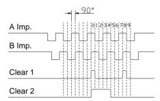
The signals Clear 1 and Clear 2 are a standard AND linked and their function can be changed through the software. See chapter "7.4.1.5.3. Inkremental-measuring system" on page 43
