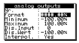
Here you enter your desired format, as described in chapter "5.4. Text input" on page 23. It is e.g. possible to make the input in percent "######" (standard), in voltage "#####V", in bar "#.###mbar" or in Ampere "##.###mA". The double-crosses are just placeholders for the real numerical values. The skaling of the input values is done in menu points "Minimum" and "Maximum".
