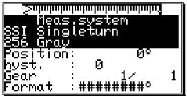
The display gives the resolution of the measuring system in steps per rotation. Generally the CamCon works with a rotation angle coder that has a resolution of 360 steps per rotation. In this case a change in the input value is superfluous. Otherwise the CamCon can be adjusted to the measuring system with the and keys. You can choose between the following
