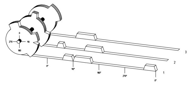
Fig.: Presentation of the principle of a cam switch unit
