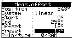
When you have entered the preset value, the device requests the input number of the preset signal with which the preset is supposed to be initiated. Enter the number next to the "P-In"-put line.
