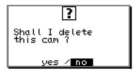
To delete the cam, move the cursor to "yes" with the key, and press the R key to confirm your choice.
