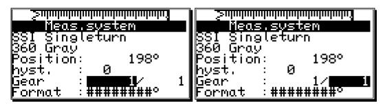
**Example:** At a full rotation of a rotation encoder with 360 steps per rotation a machine proceeds for 1000mm.
