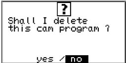
Enter the number of the program that you want to delete with the numeric keys. Press Ell and the display shows the security precaution question for the deletion of programs. Move the cursor to "ves" with the key, and press the CR key to delete the program.
