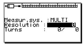
Example 1: You have a rotation plate with an electronic gear rate of 3 to 1, i.e. the encoder rotates 3 times for every rotation of the plate. These three rotations correspond with 360 impulses (360 degrees). You need to make the following inputs:
