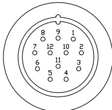
**Attention:** The order of the numbering of the connector plug may differ from manufacturer to manufacturer. You can only connect a plug with a different order, if you keep the displayed attachment allocation in mind. The location of the pins has to match the corresponding functions at the device. This booklet uses a plug of the Binder 623 series.
