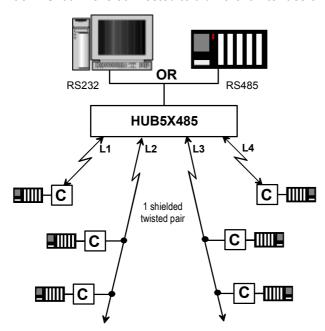
C= RS232/ RS485 converter or RS485 line isolator.
