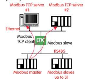
This gateway allows to connect a serial modbus master to the serial interface of the IPRS.
