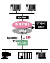
Each time a device wishes to connect to the IPL-G12, it will use its host name and get its temporary IP address from the DYNDNS server.
