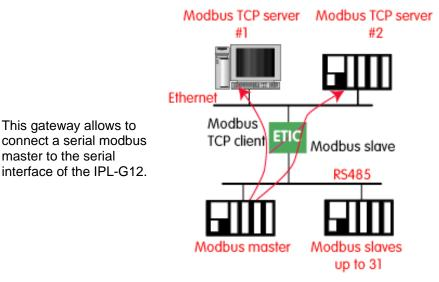
• Select the modbus menu and then "modbus client" menu; enable the "modbus client" gateway and set up the parameters as follows :
