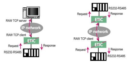
The serial device must be for example a master device in half duplex protocols.
