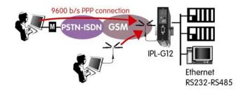
The login and password of the remote user is checked by the IPL-G12B router.
