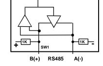
**Polarisation resistors** 1 Kohm bus polarisation resistors are included inside the product.
