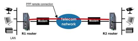
In each router, PPP connections must be set up to register the parameters of each connection (Dial number, remote LAN IP address, password ...).
