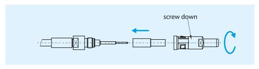
**Step 5**Assembly coax contact in insulation body
