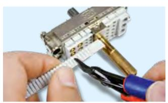
...and cut the secondary locking to length with the help of the available raster (2.4 mm).
