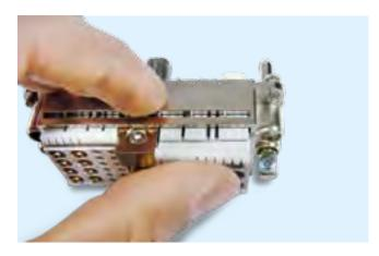
Then click the secondary lockings into the engagement hooks of the moulds.
