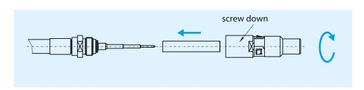
**Step 5**Assembly coax contact in insulation body
