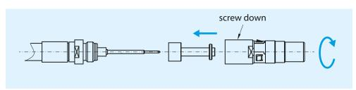
**Step 5**Assembly coax contact into insulation body
