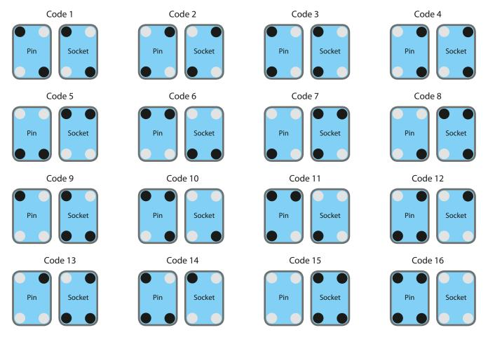
Keying order separately. Exchange screw either keying socket or keying pin! Torque value 1.25 Nm.
