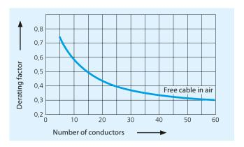
Load derating factor for plastic jacketed cable in air from 1.5 mm<sup>2</sup> to 10 mm<sup>2</sup>.
