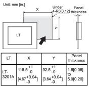
(2) Confirm that the installation gasket is attached to the LT unit and then place the LT unit into the Panel from the front.
