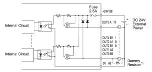
\*1 (Example) The output delay time (ON to OFF) is 1.5µs where the output current is DC 24V, 50mA. Install an external dummy resistor to increase the amount of current when more responsiveness is required and the load is light.
