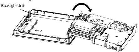
(7) Disconnect the Backlight Unit cable from the connector on the inverter board, and then remove the cable from the cable clamp.
