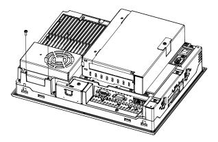
(3) Turn the fan unit upside down. Unscrew the screw (1) and lift the fan. Remove the filter between the fan cover and the fan.
