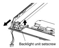
(8) Insert a new Backlight Unit while sliding it along the groove and fasten the setscrew. The necessary torque is 0.173N•m.
