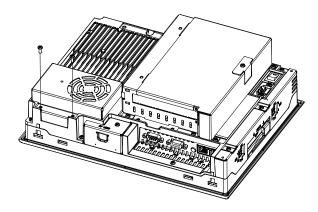
(3) Install the main memory where the following figure shows. Insert the DIM module, which is an optional product, into the connector completely in an oblique direction, then press it downward until it is locked into the stopper.
