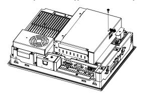
(3) Unscrew the expansion board cover's screws (2) and remove the expansion board cover.
