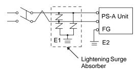
If the supplied voltage exceeds the PS-A unit's range, connect a constant voltage transformer.
