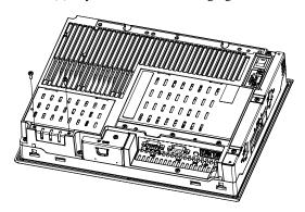
(3) Install the main memory where the following figure shows. Insert the DIM module, which is an optional product, into the connector completely in an oblique direction, then press it downward until it is locked into the stopper.
