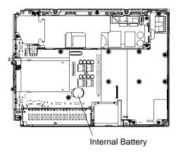
(2) Remove the battery. Push the clip of the battery holder with your finger, the forceps etc. and the battery is pushed up and removed.
