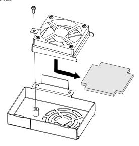
(4) Remove dust on the filter using a cleaner etc. If stubborn dirt or stains are present, wash the filter with a neutral detergent.
