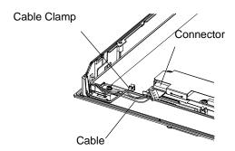
(7) Loose the Backlight Unit setscrew (1), and lift the edge of the Backlight Unit, and remove the unit while sliding it along the groove.
