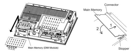
(4) Place back the Memory slot cover and fix with two screws. The torque required to tighten these screws is 0.5 to 0.6N•m.
