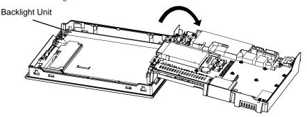
(6) Disconnect the Backlight Unit cable from the connector on the inverter board, and then remove the cable from the cable clamp.
