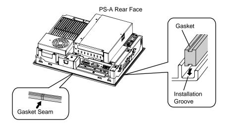
(4) Check that the gasket is attached correctly to the PS-A. The upper surface of the gasket should protrude approximately 2 mm [0.08 in.] out of the groove evenly.
