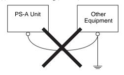
• When supplying power to the PS-A unit, be sure to separate the input/output and power lines, as shown. [diagram (a)]
