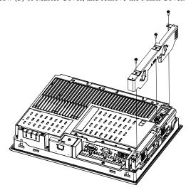
(4) Unscrew the screws (6) (See the figure below).
