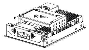
(6) Place back both of the expansion board cover and expansion board support. The torque required to tighten each of the screws is 0.5 to 0.6N ⋅ m.
