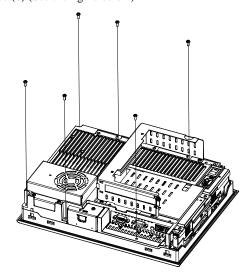
(6) Open the PS-A unit as the figure below indicates.
