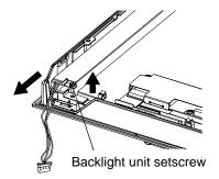
(9) Insert a new Backlight Unit while sliding it along the groove and fasten the setscrew. The necessary torque is 0.173N•m.
