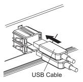
(3) Insert the USB cover into the tab of the USB holder to fix the USB cable.
