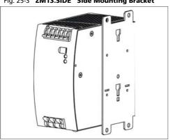
Fig. 25-4 Side Mounting with DIN-rail brackets
