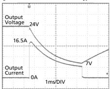
Peak load 16.5A (resistive) for 5ms Output voltage dips from 24V to <u>7V.</u>
