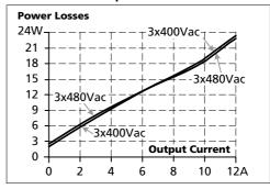
Fig. 10-4 Losses vs. input voltage, 24V, 10A, 3-Phase Operation
