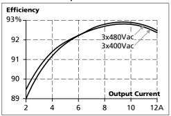
Fig. 10-3 Efficiency vs. input voltage, 24V, 10A, 3-Phase Operation
