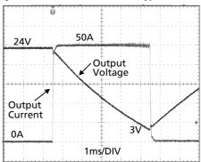
Peak load 50A (resistive) for 5ms Output voltage dips from 24V to 3V.
