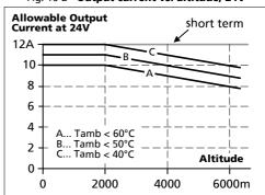
The ambient temperature is defined as the air temperature 2cm below the unit.
