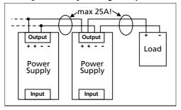
Fig. 26-11 Using distribution terminals
