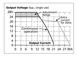
Fig. 8-2 Output voltage in "parallel use mode", typ.
