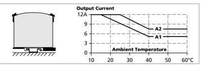
Fig. 26-16 Mounting Orientation D (Horizontal cw)
