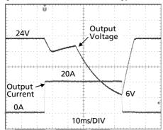
Peak load 20A (resistive) for 50ms Output voltage dips from 24V to 6V.
