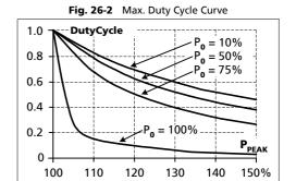
$$D_{uty}C_{ycle} = \frac{T_{peak}}{T_{peak} + T_0}$$
