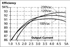
Fig. 11-3 Efficiency vs. input voltage, 24V, 5A
