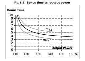
Bonus Power<sup>®</sup> is available as soon as power comes on and immediately after the end of an output short circuit.
