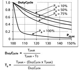
Fig. 27-2 Max. Duty Cycle Curve
