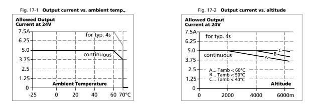
The ambient temperature is defined as the air temperature 2cm below the unit.
