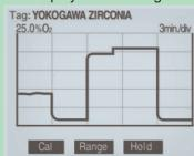
During automatic calibration, you can check stabilized display data while viewing oxygen trend data, thus providing highly reliable calibration.
